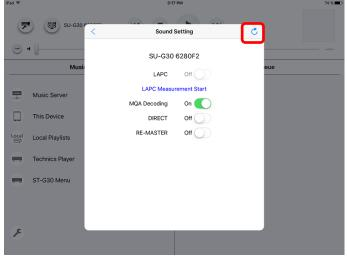
· "MQA" or "MQA Studio" indicates that the unit is decoding and playing an MQA stream or file, and denotes provenance to ensure that the sound is identical to that of the source
